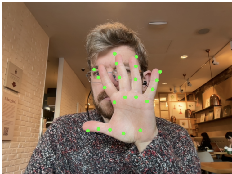
Figure 4: Hand detection live via webcam. The circles mark points on the palm and fingers. It's not perfect but it's pretty quick!
