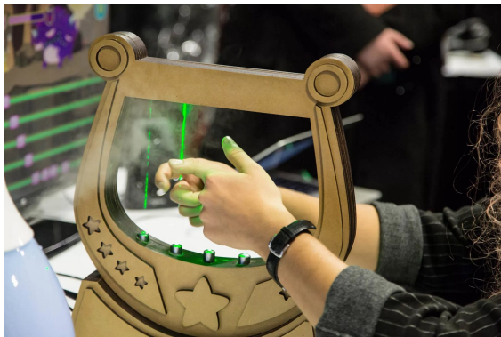
(c) Orpheus Quest, an alt controller using motion sensors built into a fake harp.
